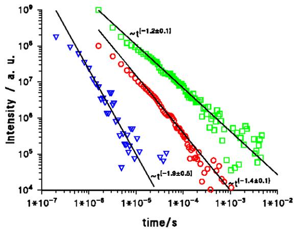
Figure 3. Decay of the violet luminescence of AlN at 5 K: Triangles: Photoluminescence of AlN on sapphire (sample LS005: 400 nm MBE-ALN on  $\text{Al}_2\text{O}_3$ ) at 400 nm, Circles: Cathodoluminescence of AlN on sapphire (sample LK48: 600 nm MOCVD-ALN on  $\text{Al}_2\text{O}_3$ ) at 423 nm Squares: Cathodoluminescence of AlN on SiC (sample LS12: 575 nm MBE-ALN on SiC) at 355 nm. The measurements were done at the maximum intensity wavelength.
