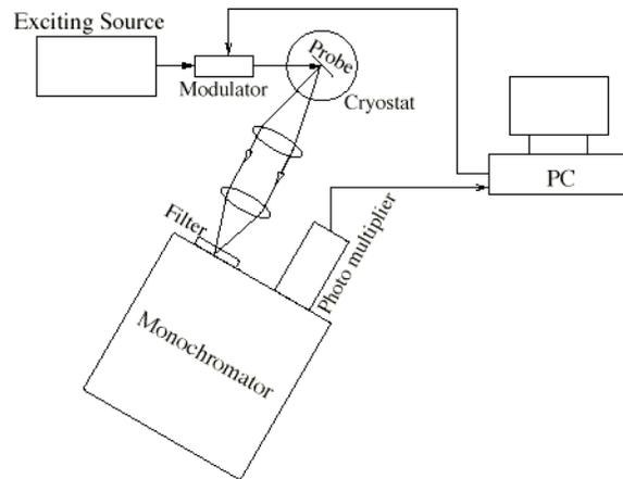
Figure 1. Breadboard construction with the correlation method
